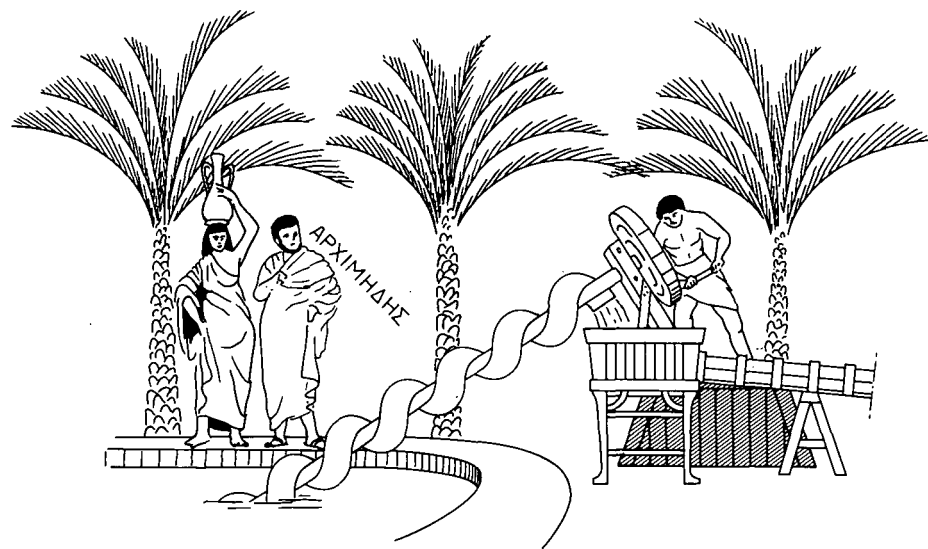
Figure 23.1 The ancient Archimedean screw
